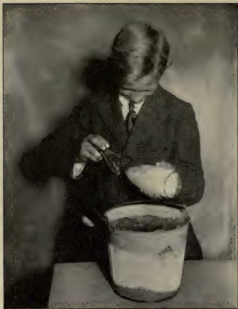
FIG. 47. Why did the bottle break when the water in it turned to ice?
